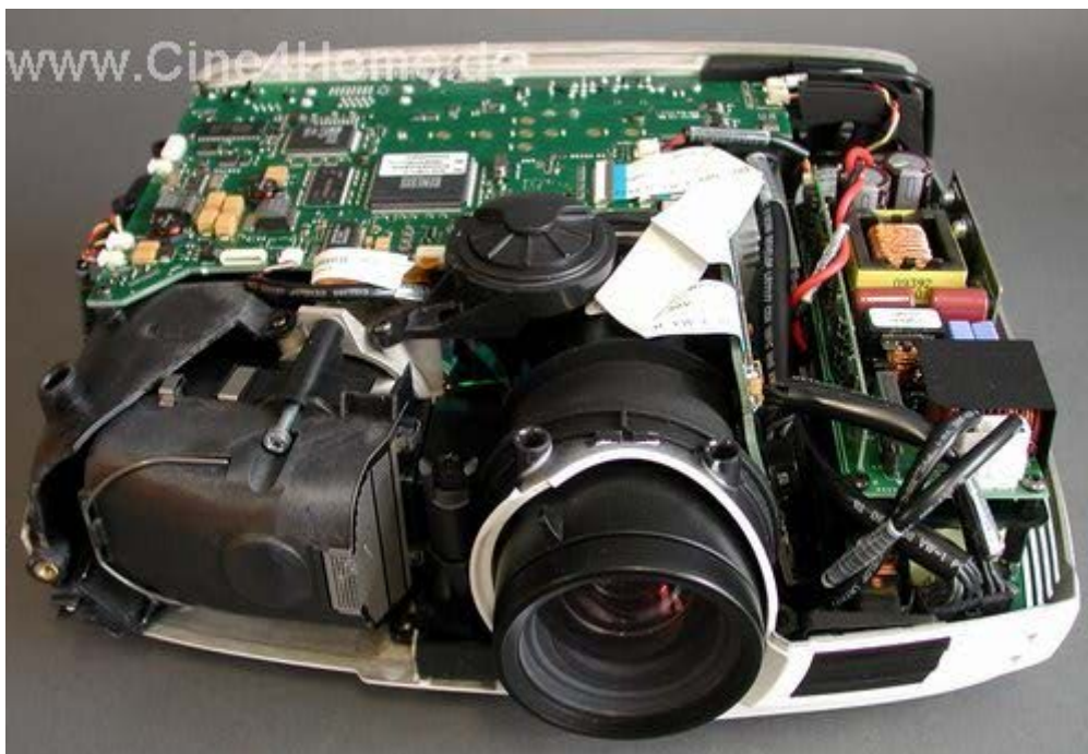
Action! model two ohne schirmenden Metall-Deckel
